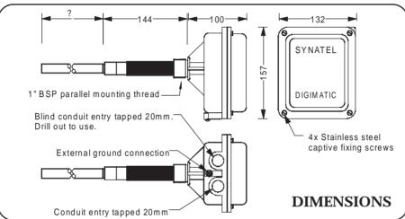
Auto-calibrating, Fixed Point, Capacitance Level Sensor with digital settings display DML4
