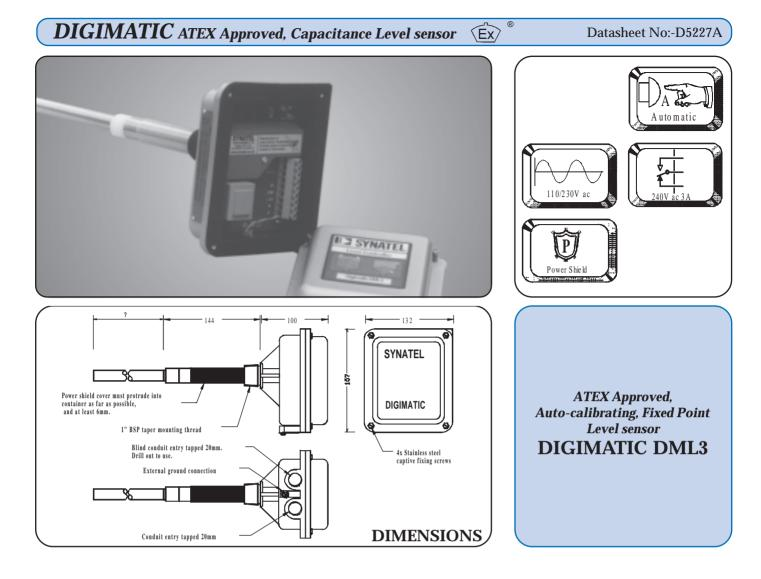
A certified, automatic calibration level control for use in liquids, solids and powders. *Certified to ATEX,* group II, Category 1,Dust, Temperature  $T80^{\circ}C$ . (M101528A  $\langle E_X \rangle$  II 1D T80°C BAS99ATEX1275).
