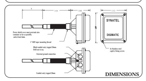
Autocalibrating, Fixed Point, Capacitance Level Sensor DIGIMATIC - DML2
