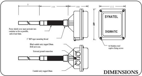
Autocalibrating, Fixed Point, Capacitance Level Sensor DIGIMATIC - DML1
