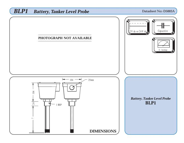
The BLP1 battery, tanker level probe has been specially designed for remote applications, typically in vehicle installations, for use in conductive or non-conductive liquids.
