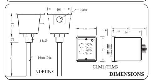
Modular Continuous Capacitance Level Sensor CLM1 - NDP1/INS
