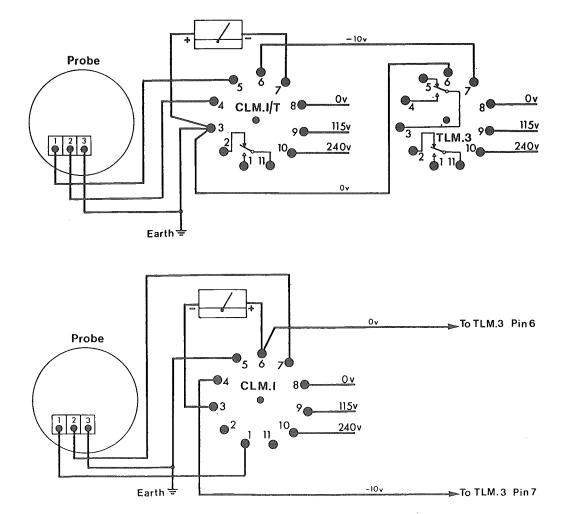
6. On the TLM.3 module the upper control relates to the relay contacts wired to Pins 3, 4 and 5 and the lower control to the contacts wired to Pins 11, 1 and 2. The upper control relay is normally de-energised and energises at trip point or above, the lower control relay is normally energised and de-energises at trip point or above. The associated LED indicators are illuminated when the relays are energised.
