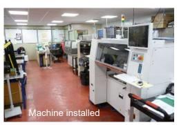
A major investment programme has been implemented within Synatel. A new additional surface mount machine, for automatically placing electronic components, has been installed. The production department and design department have all had a major make-over, and it is intended that the Test department is also improved and new servers installed to maintain reliability.
